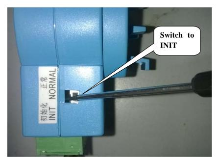
**2.** put switch to INIT, then connect the power
